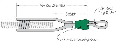
The Steel Dog® Cam-Lock Loop-Coil™ Tie is a multipurpose Transition Tie™. With loop tie end and self centering cone, electronically welded to a two-strut, ½"coil tie end, the Cam-Lock Loop-Coil™ Tie allows the user to take advantage of the versatility of threaded coil rod for one-sided forming, long ties, and other purposes, when using Gates Cam-Lock forms and hardware.
