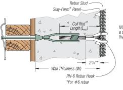
NOTE: Rebar Hook has a different load rating than Snap-Coil Ties.
