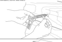
•Screw into wood using impact wrench or socket driver on bolt hex head (400 ft-lb torque MAX).If excessive resistance is met, unscrew bolt and re-lubricate
