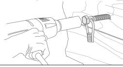
•Thread desired length of  $\frac{1}{2}$ "coil rod or  $\frac{1}{2}$ "-13 rod into swivel loop coil
