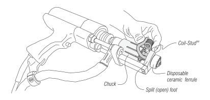
Steel Dog<sup>®</sup> **Coil-Studs**<sup>™</sup> can be welded with the same setup used for 3/4" shear connectors. Switching between the two is simply a matter of adjusting the length between the ferrule foot and the chuck.
