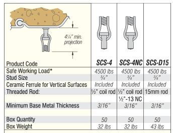
\*For Coil-Stud itself at approximately 2-to-1 Safety Factor. ACTUAL ALLOWABLE LOAD WILL DEPEND ON INSTALLATION AND STRENGTH OF WELD.
